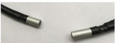
Push together and seal with PVC tape
